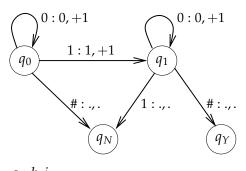
Here something like (q) a: b, i (q') means: when in state q and reading symbol a, change to state q', write symbol b and move the tape head by the increment i.
