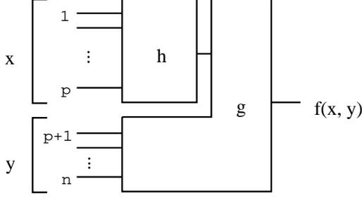
**Figure 1. Simple disjunctive decomposition**
