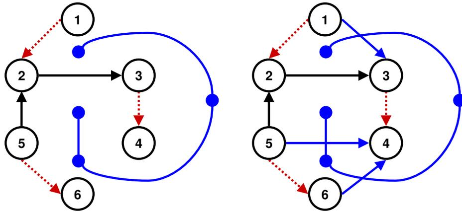
**Figure 5.2** The left graph is the spanning tree  $T$  for  $G_6$  together with the blue tree,  $T'$ , which has the vertex set of the dual of  $G_6$ . On the right,  $T$  is completed to  $G_6$  such that  $G_6$  is now Pfaffian. By redirecting the original edge  $(3, 1)$  the only sign-switching cycle of  $G_6$  is now oddly oriented.
