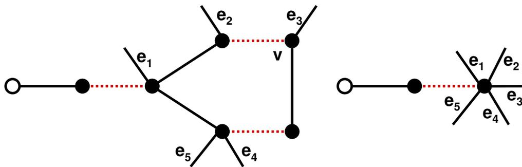
**Figure 4.1** The left graph starts from the free vertex followed by a black (unmatched) edge not in  $M$ ; red dashed (matched) edges are in  $M$ . The stem leads to the blossom which is then contracted into a super vertex; see the right graph.
