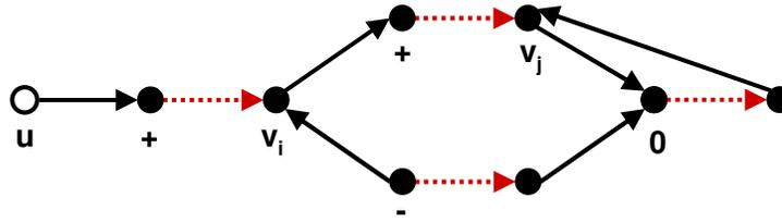
**Figure 6.8** One branch of the sign neutral path is revisited, changing the status of the “0” vertex. This forms a blossom at  $v_j$  which is contracted into  $b_1^*$ , which then creates another blossom starting at  $v_i$ . This destroys the “0” state because part of the path is needed to construct the augmenting path.
