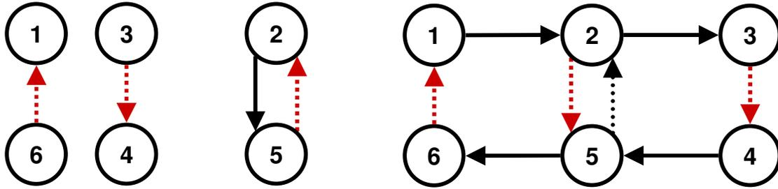
**Figure 5.4** Find a perfect matching in  $G - G^*$ , the leftmost graph, given by edges  $(6,1)$  and  $(3,4)$ . There is only one such perfect matching, which has odd sign. In  $G^*$  there exists a perfect matching of either sign, we pick edge  $(2,5)$ , which has positive sign. Combining the two perfect matching gives a negative signed perfect matching of  $G$  at  $M' = \{(6,1)(2,5)(3,4)\}$ .
